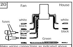
Make wiring connections as indicated above. White from fan to white from remote marked N. Orange from fan to Orange from remote marked Light/up. Blue from fan to blue from remote marked down light. Black from fan to Black from remote marked L. White from house to white from remote marked AC N. Black from house to Black from remote marked AC L. Connect all green ground wires to Ground wire from House.
